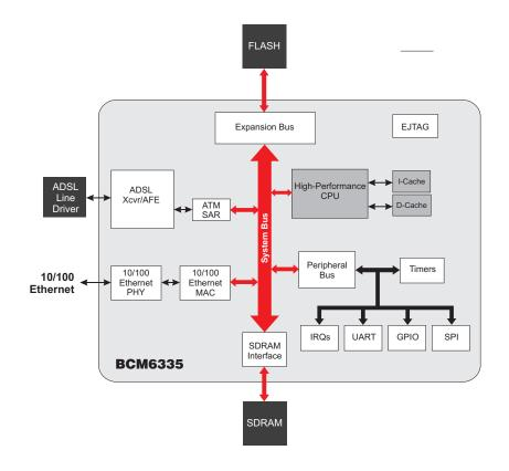
The **BCM6335** is a single-chip G.992.1/G.992.2/G.992.3 and T1.413 ADSL-to-Ethernet CPE router with a high-performance MIPS32<sup>™</sup> CPU, a 10/100-Mbps Ethernet interface with Auto-MDIX, and FLASH and SDRAM interfaces.
