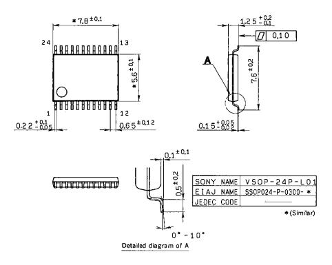
Note) Dimensions marked with \* do not include resin residue.
