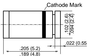
Dimensions are in inches and (millimeters)
