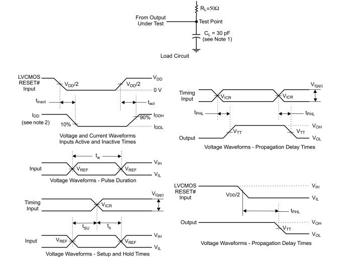
Parameter Measurement Information ( $V_{DD} = 2.5V \pm 0.2V$ )
