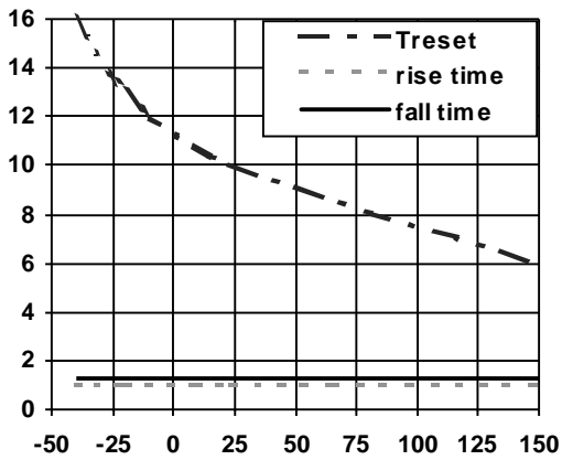
Figure 18 - Rise Time, Fall Time and Treset (µs) Vs Tj (°C)
