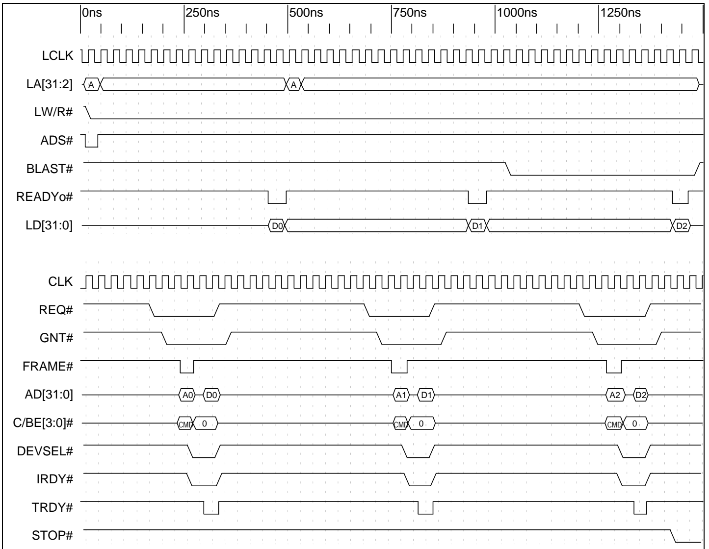
Timing Diagram 8-40. (C Mode) Local Bus Direct Master Read from PCI I/O
