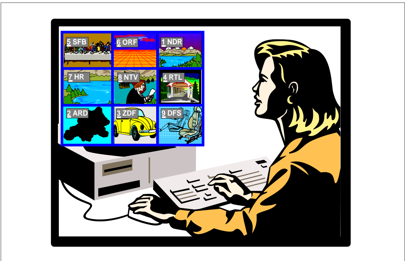
Figure 7 Multi-PIP Feature with Display Mode 7 Main picture and one PIP picture live, all other pictures still
