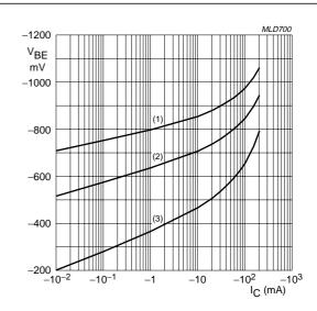
**TR2 (PNP)**;  $V_{CE} = -5 \text{ V}$ .
