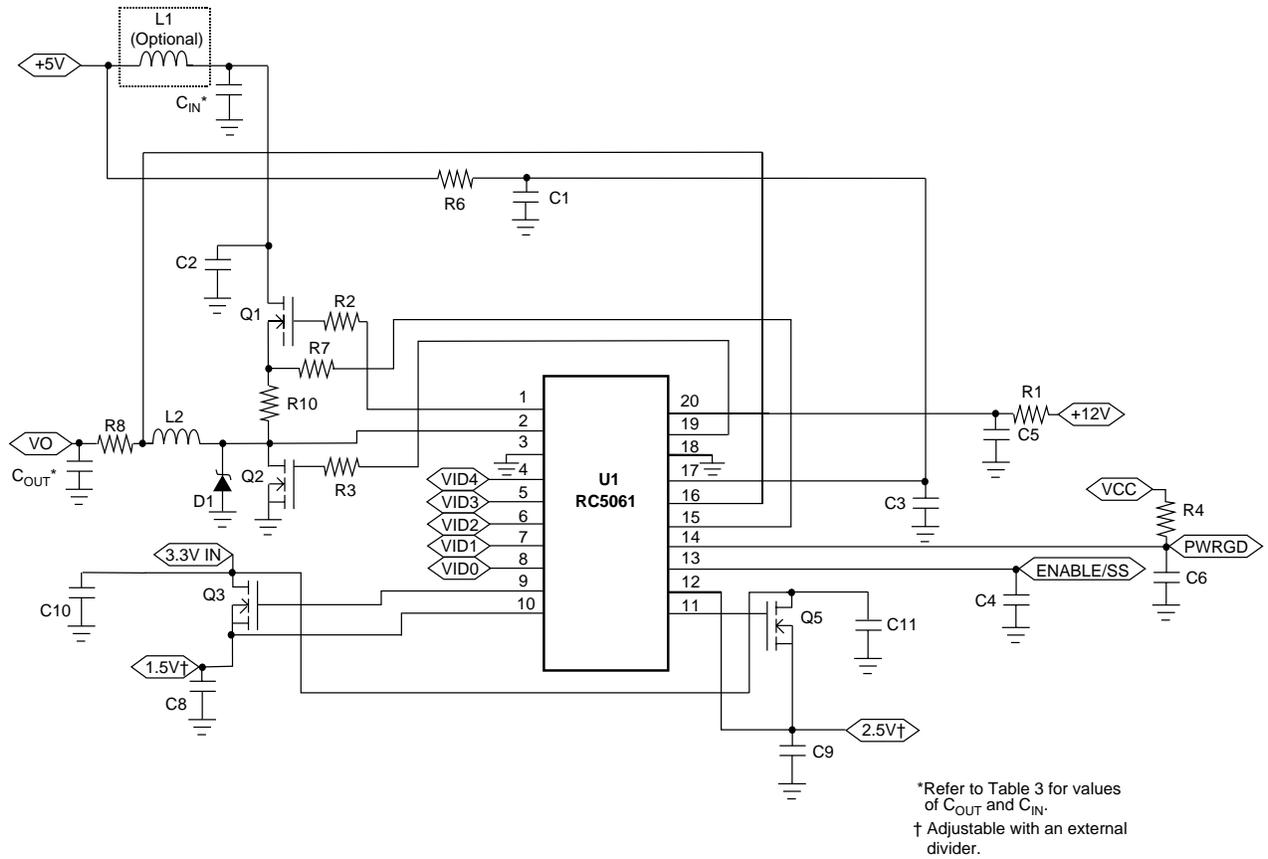
Figure 2. Application Circuit for Coppermine/Camino Motherboards
