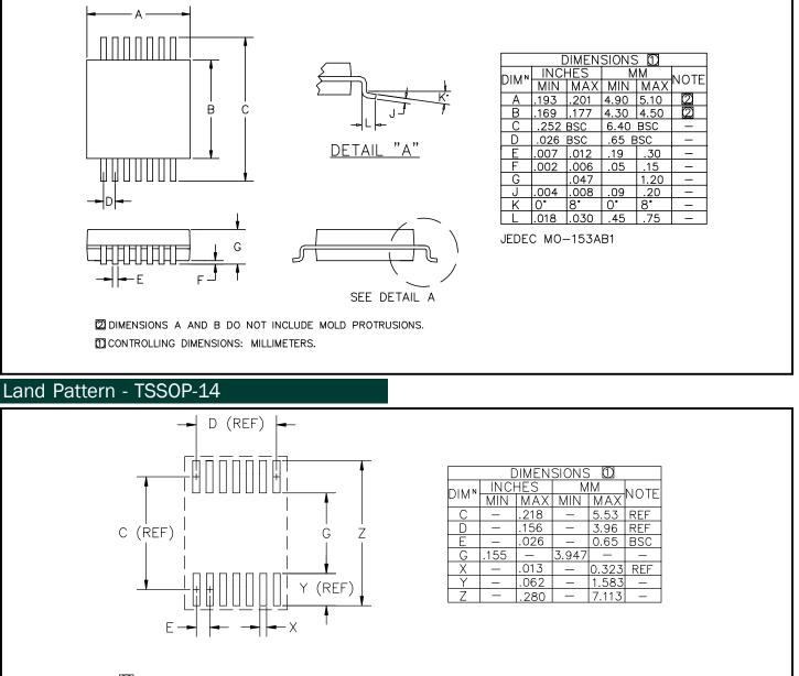
GRID PLACEMENT COURTYARD IS 10 X 15 ELEMENTS (5mm X 7.5mm) IN ACCORDANCE WITH THE INTERNATIONAL GRID DETAILED IN THE IEC PUBLICATION 97.
