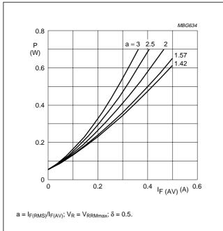
Fig.4 Maximum steady state power dissipation (forward plus leakage current losses, excluding switching losses) as a function of average forward current.
