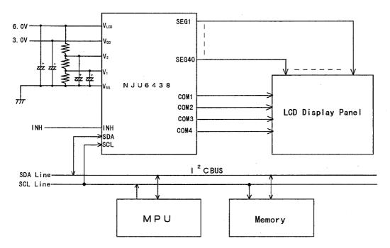
(Note) The internal display data is undefined when  $V_{\text{DD}}$  is just turned on.
