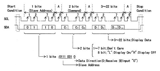
Whole 160bits data transfer to the shift register. When the input data in less than 160 bits, parts which bit data is inputed corresponded to display, and segment which correspond to the rest part in "off".
