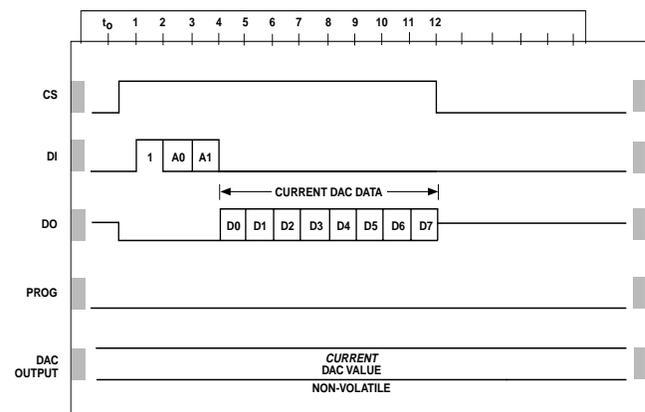
this value is the same as that which had been there previously no change in the DAC's output is noticed. Had the value held in the control register been different from that stored in EEPROM then *a change would occur* at the read cycle's conclusion.
