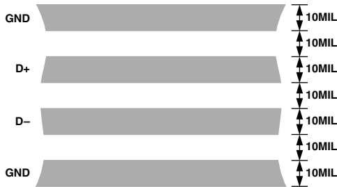
Figure 4. Arrangement of Signal Tracks
