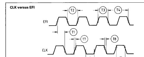
The EFI input low and high times as shown are required to guarantee the CLK low and high times shown.
