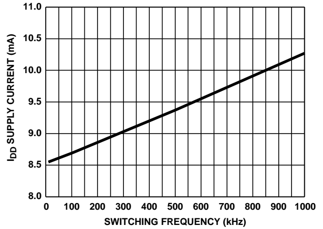
FIGURE 5. I DD0 , NO-LOAD I DD SUPPLY CURRENT vs FREQUENCY (kHz)
