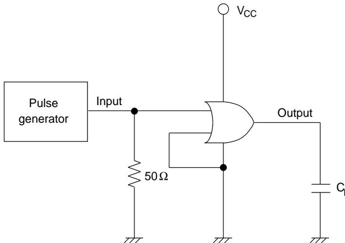
Note: Operating current test time, output is open.
