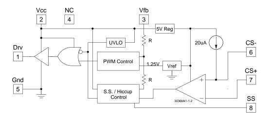
Figure 1 - Simplified block diagram of the US3036
