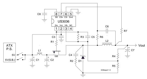
Figure 2- The circuit in figure 2 is the application of the US3036 providing a low cost solution for a 2.5V supply from the 5V dual supply.
