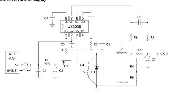
Figure 2- The circuit in figure 2 is the application of the US3036 providing a low cost solution for a 2.5V/2A supply from the 5V dual supply. This circuit uses current sense resistor to set the current limiting.
