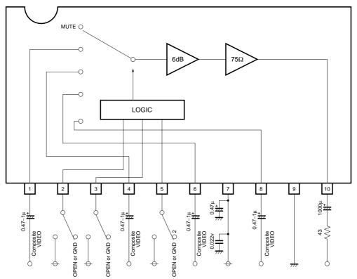
\*The output impedance has  $32\Omega$ , please use  $43\Omega$  resistor for outside matching.
