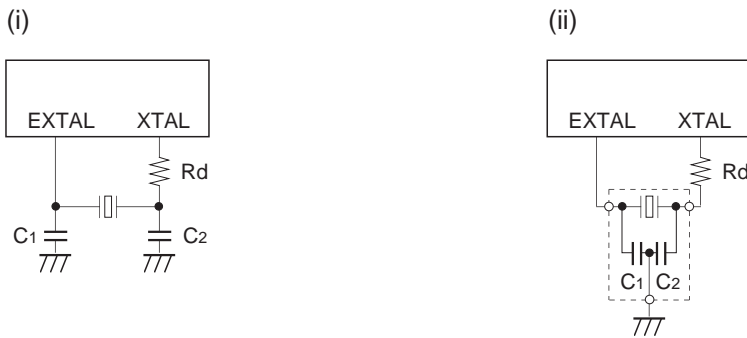
Fig. 13. Recommended oscillation circuit
