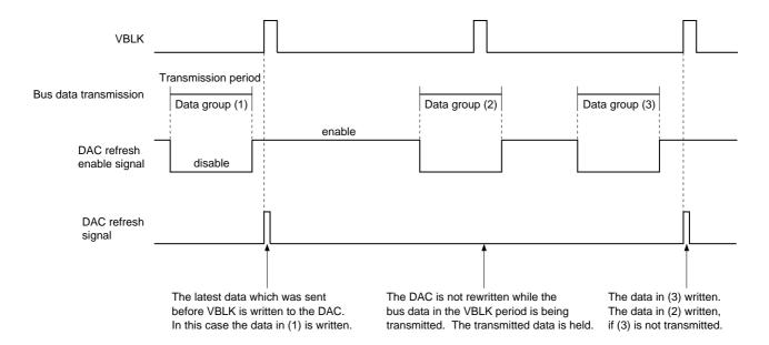
The VBLK signal is extracted from the composite BLK signal which has been input to Pin 14, and the DAC data for each control is rewritten all at once in synchronization with this VBLK signal. The received I<sup>2</sup>C bus data is held by a latch until the next VBLK signal arrives. Therefore, I<sup>2</sup>C bus data transmission from the microcomputer is timing-free. Set the width of the V blanking pulse which is input to Pin 14 to 300µs or more.
