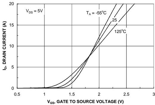
Figure 5. Transfer Characteristics.
