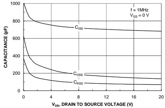
Figure 8. Capacitance Characteristics.
