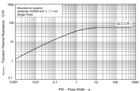
TRANSIENT THERMAL RESISTANCE vs. PULSE WIDTH
