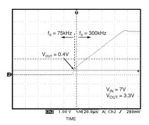
Figure 4. Startup Waveform
