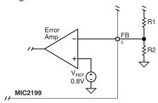
Figure 6. Voltage-Divider Configuration
