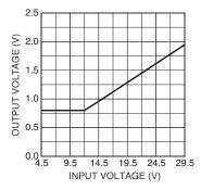
Figure 5. Minimum Output Voltage vs. Input Supply Voltage
