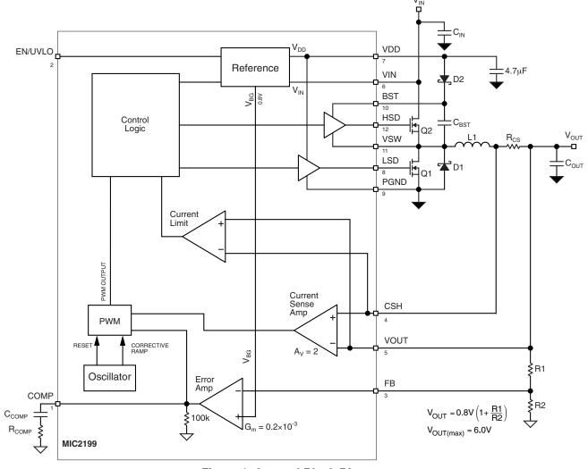
Figure 1. Internal Block Diagram
