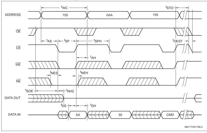
Notes: (6) The Store Pulse Width ( $t_{SP}$ ) is a minimum time that  $\overline{NE}$ ,  $\overline{WE}$  and  $\overline{CE}$  must be LOW simultaneously. (7)  $t_{SOE}$ ,  $t_{OEST}$  and  $t_{NHZ}$  are periodically sampled and not 100% tested.
