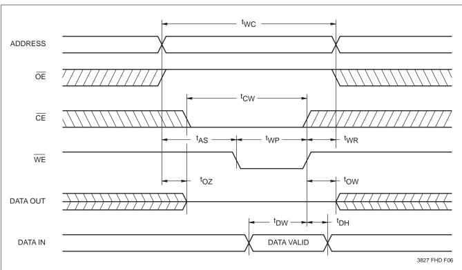
$\textbf{Note:} \quad \text{(4)} \ \ \, t_{WZ},\, t_{OW} \text{ and } t_{OZ} \text{ are periodically sampled and not 100\% tested.}$
