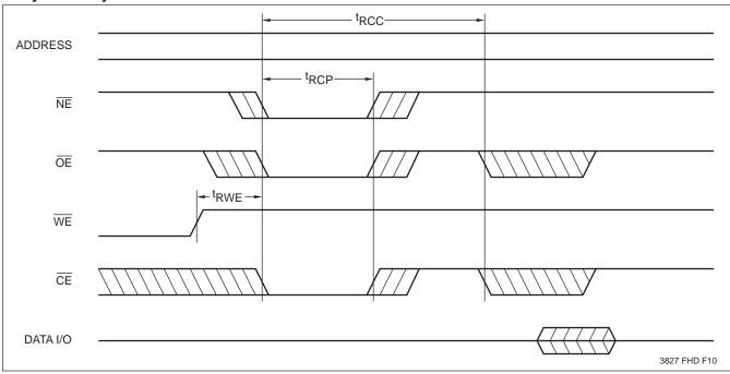
Note: (5) The Recall Pulse Width  $(t_{RCP})$  is a minimum time that  $\overline{NE}$ ,  $\overline{OE}$  and  $\overline{CE}$  must be LOW simultaneously to insure data integrity,  $\overline{NE}$  and  $\overline{CE}$ .
