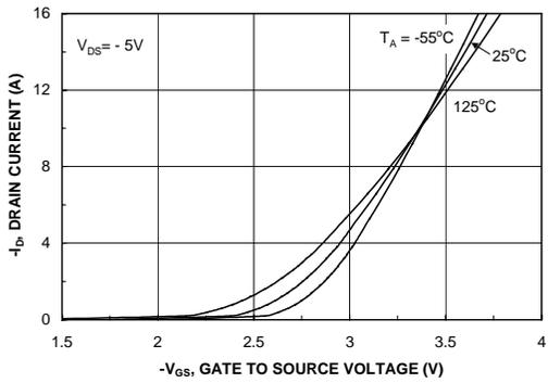
Figure 5. Transfer Characteristics.
