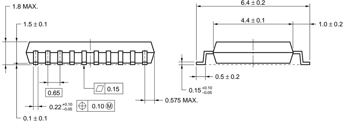
**NOTE** Each lead centerline is located within 0.10 mm of its true position (T.P.) at maximum material condition.
