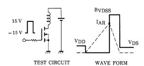
$$\begin{aligned} R_G &= 25~\Omega,~V_{DD} = 90~V \\ L &= 12.2~mH \end{aligned} \qquad E_{AS} = \frac{1}{2} \cdot L \cdot I^2 \cdot \left( \frac{BVDSS}{BVDSS - V_{DD}} \right) \end{aligned}$$
