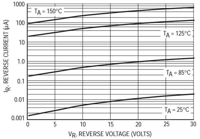
**Figure 3. Leakage Current**
