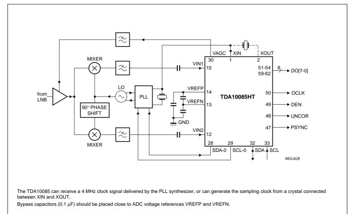
Fig.3 Front-end receiver schematic.
