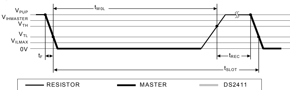
Figure 7c. Read-data Time Slot
