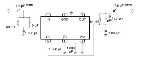
Note Matching can be adjusted with trimmer condenser.
