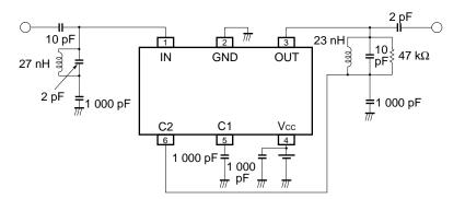
ILLUSTRATION OF THE TEST CIRCUIT 4 ASSEMBLED ON EVALUATION BOARD
