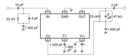
ILLUSTRATION ON THE TEST CIRCUIT 6 ASSEMBLED ON EVALUATION BOARD
