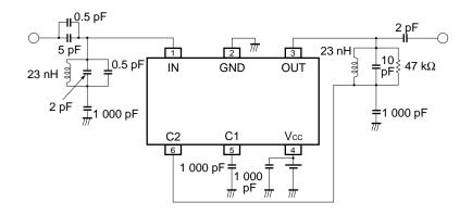
ILLUSTRATION OF THE TEST CIRCUIT 3 ASSEMBLED ON EVALUATION BOARD
