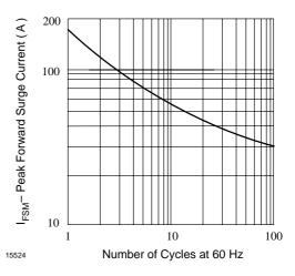
Figure 3. Max. Peak Forward Surge Current vs. Number of Cycles
