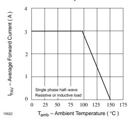
Figure 1. Max. Average Forward Current vs.
