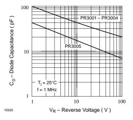
Figure 4. Typ. Diode Capacitance vs. Reverse Voltage
