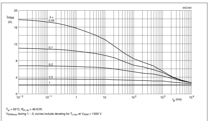
Fig.4 Maximum repetitive peak forward current as a function of pulse time (square pulse) and duty factor.
