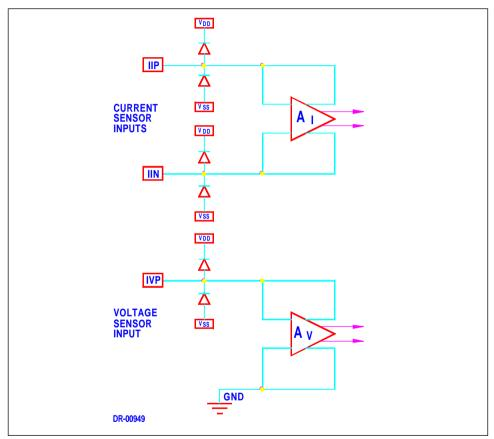
**3.** Electrostatic Discharge (ESD) Protection The SA9105F integrated circuit's inputs/outputs are protected against ESD.
