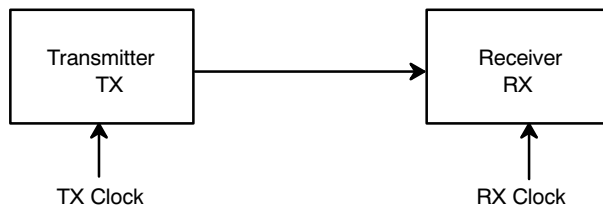
Figure 29. Example of a Serial Data Transmission System
