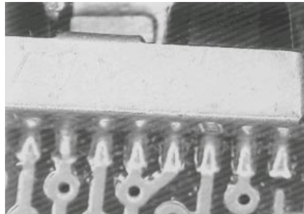
Photo 4.0. Unit self-aligns after reflow.
