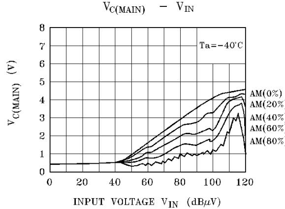
IC temperature characteristics (Measure the temperature characteristics of the IC by using the resistor instead of the resonant circuit.)
