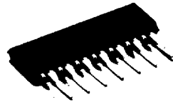
Outline 14P5A(L) 1.27mm pitch 325mil ZIP (2.8mm × 19.0mm × 6.3mm)
