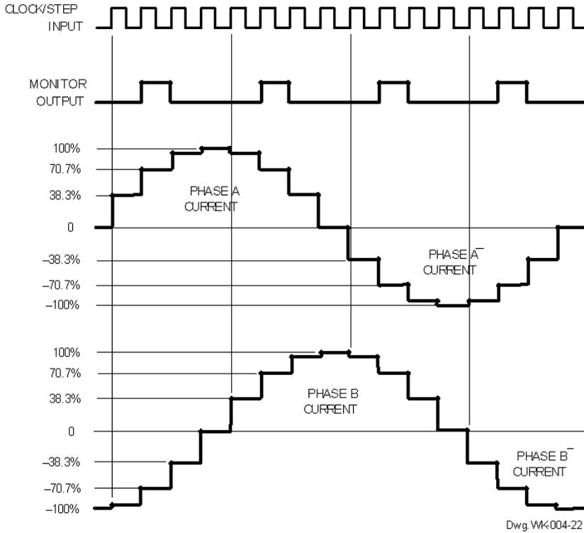
Quarter-step output current waveshapes (all devices). For illustrative purposes, phase A\ or B\ current (unipolar drive) is shown as negative current.
