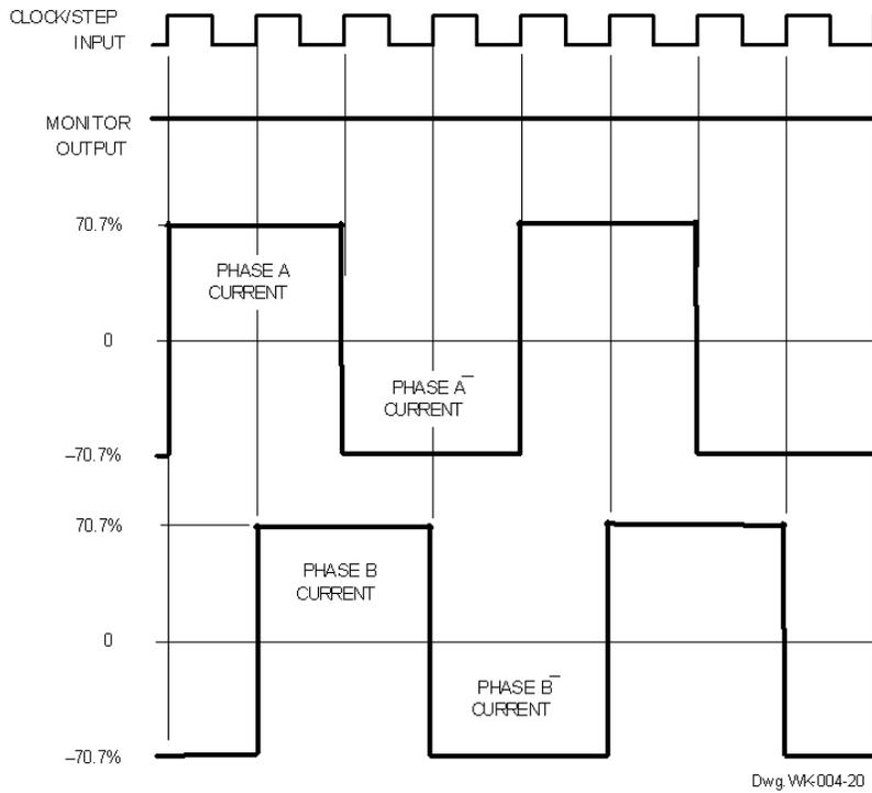
Full-step (2-phase) output current waveshapes (SLA7065/66/67M only). For illustrative purposes, phase A\ or B\ current (unipolar drive) is shown as negative current.
