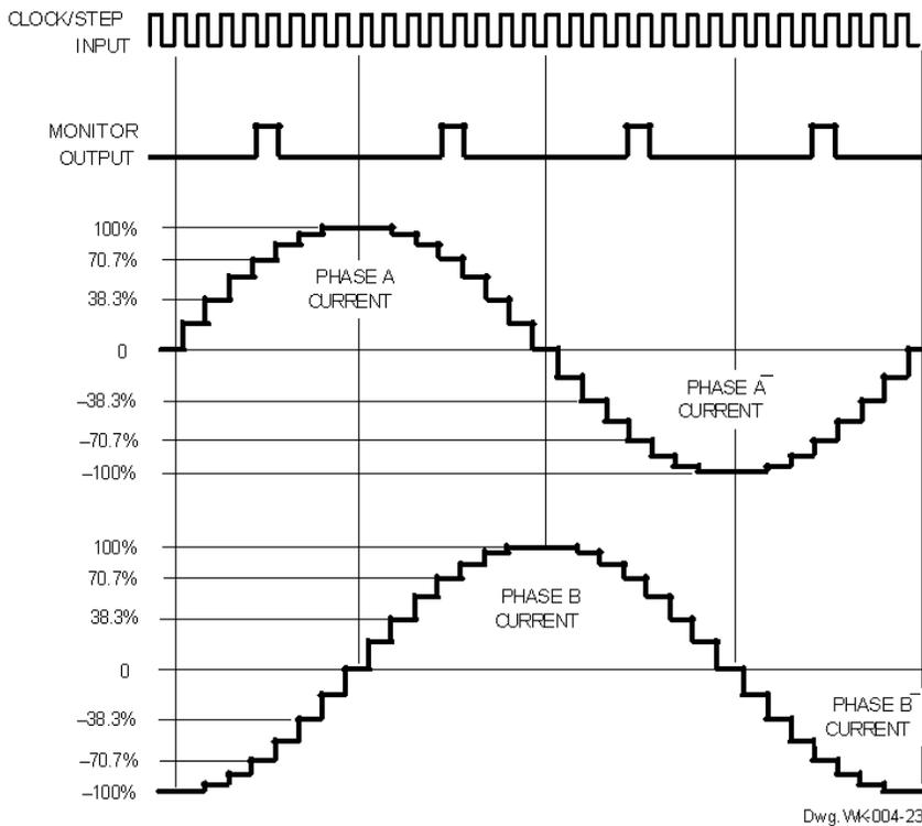
Eighth-step output current waveshapes (all devices). For illustrative purposes, phase A\ or B\ current (unipolar drive) is shown as negative current.
