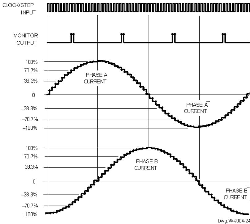
Sixteenth-step output current waveshapes (SLA7060/61/62M only). For illustrative purposes, phase A\ or B\ current (unipolar drive) is shown as negative current.
