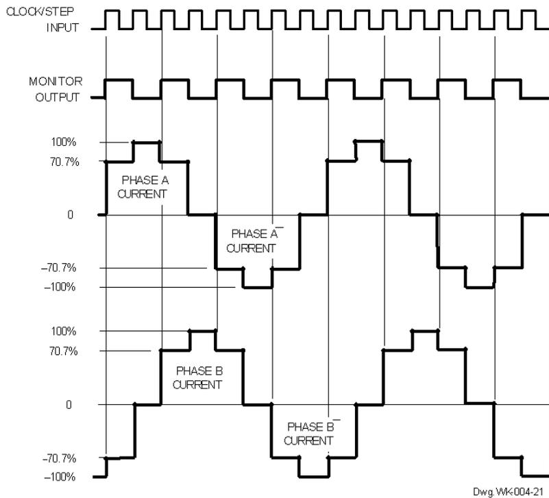
Half-step output current waveshapes (all devices). For illustrative purposes, phase A\ or B\ current (unipolar drive) is shown as negative current.
