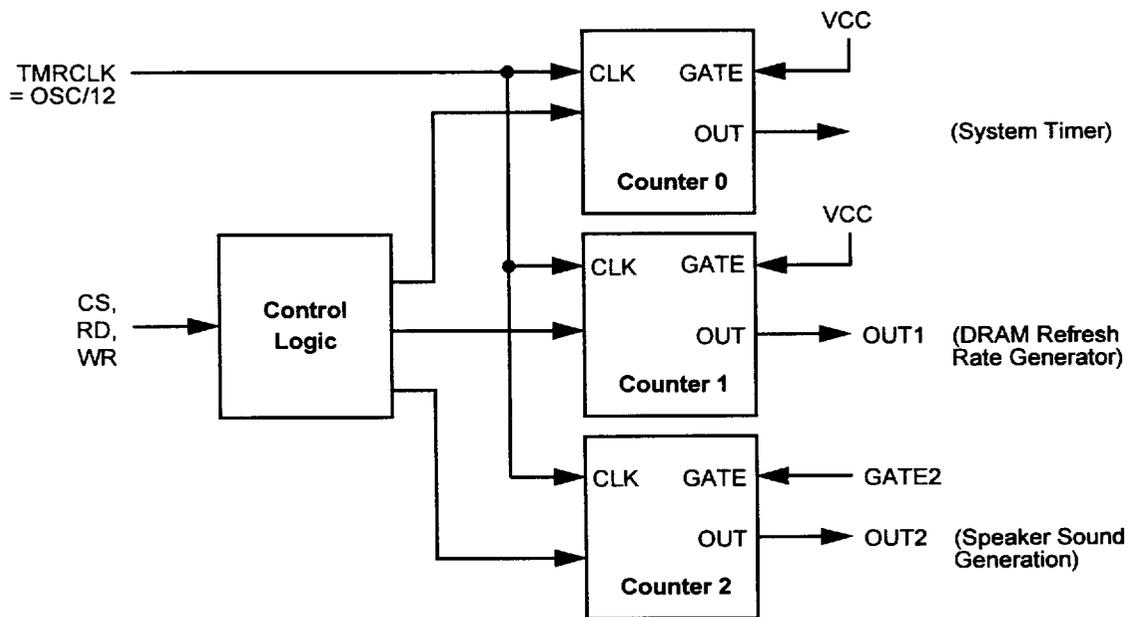
The 16-bit counting component is a loadable synchronous down counter. It is loaded or decremented on the falling edge of TMRCLK. The counting component contains a maximum count when a 0 is loaded, which is equivalent to 65536 in binary operation or 1000 in BCD. The counting component does not stop when it reaches 0. In Modes 2 and 3, the counting component will be reloaded and in all other modes it will wrap around to 0FFFFh in binary operation or 9999 in BCD.
