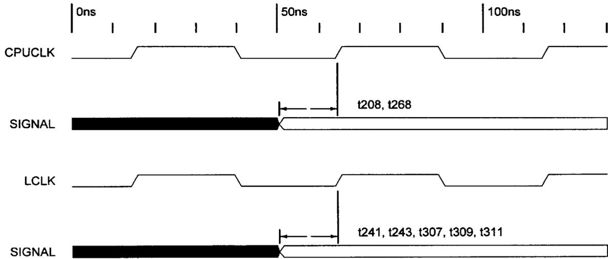
Figure 6-3 Output Delay Timing Waveform
