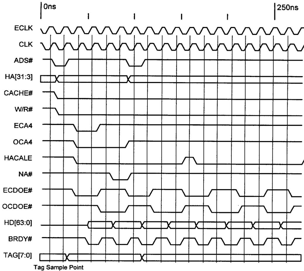
Figure 4-5 L2 Cache Read Hit Cycle - Sync. SRAMs
