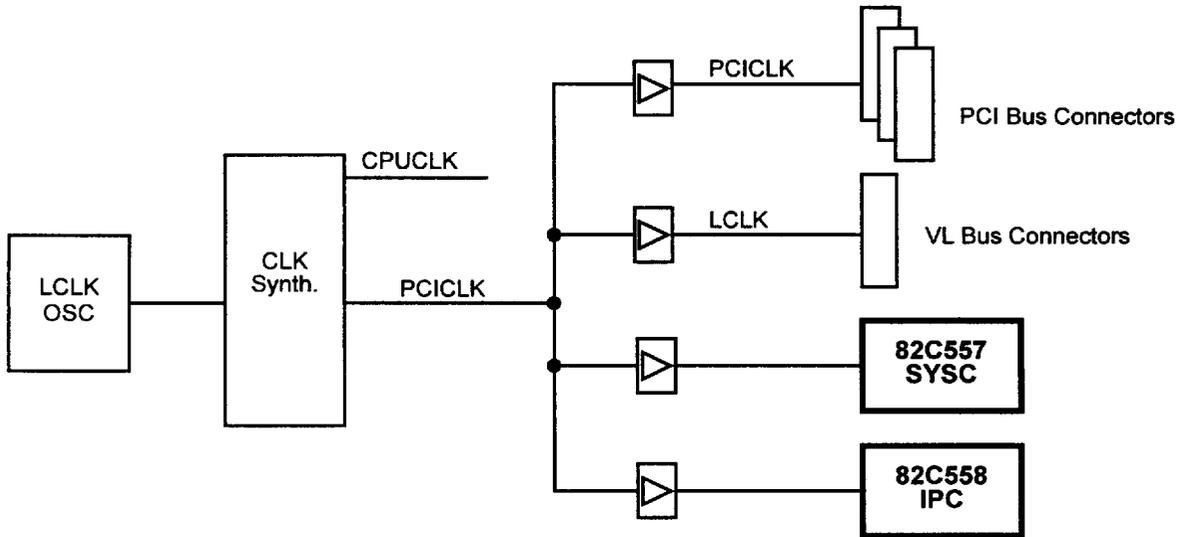
**Figure 4-3 Clock Distribution Method for VL Bus and PCI Connectors (Sync. PCI and VL Bus)**
