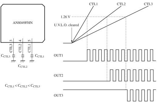
Figure 8. Sequential operation
