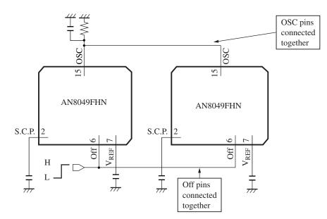
Figure 7. Slave operation circuit example
