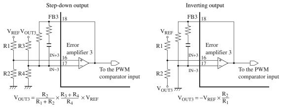
Figure 4. Connection method of error amplifier 3
