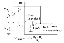
Figure 2. Connection method of error amplifier 1 (Step-up output)
