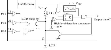
Figure 6. Short-circuit protection circuit
