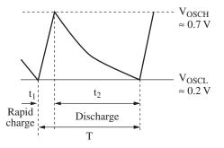
$f_{OSC} \approx -\frac{1}{C_{T} \times R_{T} \times \ln \frac{V_{OSCL}}{V_{OSCH}}} \approx 0.8 \times \frac{1}{C_{T} \times R_{T}}$ (Hz)
