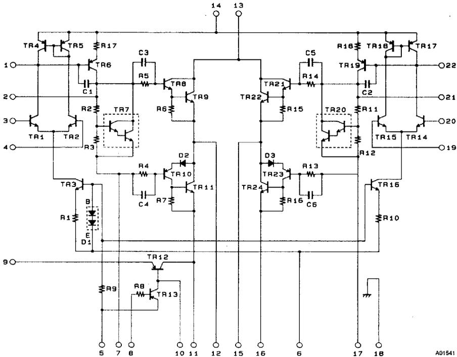
Sample Application Circuit (100W min 2-Channel AF Power Amplifier)
