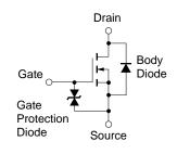
The diode connected between the gate and source of the transistor serves as a protector against ESD. When this device acutally used, an additional protection circuit is externally required if voltage exceeding the rated voltage may be applied to this device.
