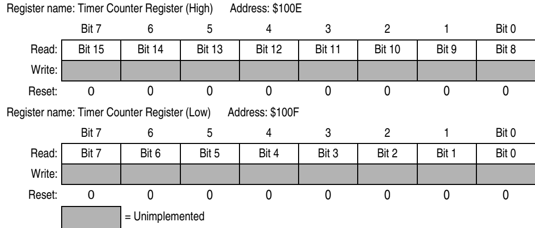
Figure 9-15. Timer Counter Register (TCNT)
