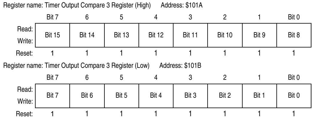
Figure 9-10. Timer Output Compare 3 Register Pair (TOC3)
