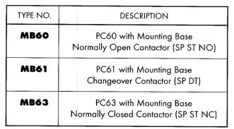
All versions of "PC" contactors can be supplied with a separate mounting base which can be soldered to the circuit board.
