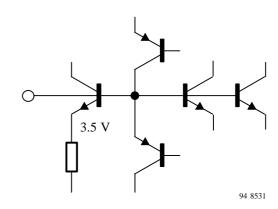
Figure 15. Internal reference voltage (Pin 17)
