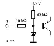
Figure 6. Input selector switch (Pin 3)
