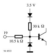
Figure 17. AFC switch (Pin 19)
