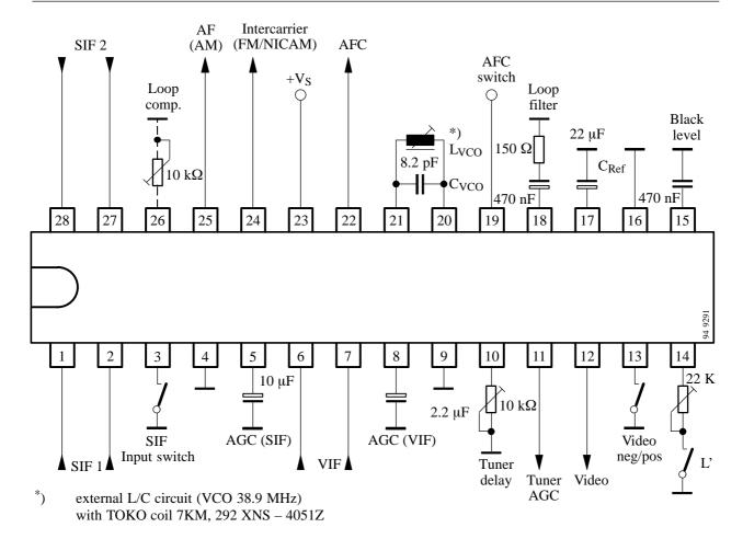
Figure 3. Test circuit
