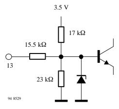
Figure 13. Standard switch (Pin 13)
