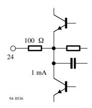
Figure 20. Intercarrier output (Pin 24)
