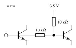
Figure 22. VCO offset compensation (Pin 26)
