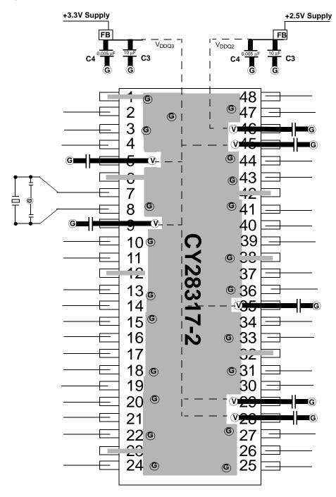
FB = Dale ILB1206 - 300 (300 $\Omega$  @ 100 MHz) or TDK ACB2012L-120 Ceramic Caps C3 = 10–22  $\mu$ F C4 = 0.005  $\mu$ F C6 = 0.01  $\mu$ F
