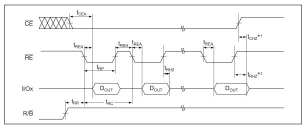
Note: 1. The time until it becomes Hi-Z depends on the earliest signal which  $\overline{\text{CE}}$  and  $\overline{\text{RE}}$  go to high.
