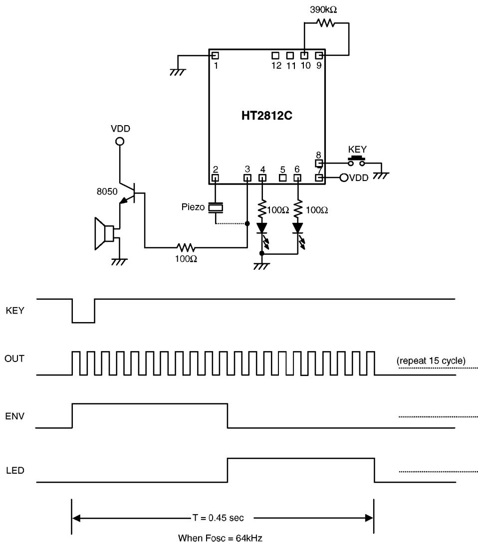
\* The IC substrate should be connected to VDD in the PCB layout artwork.
